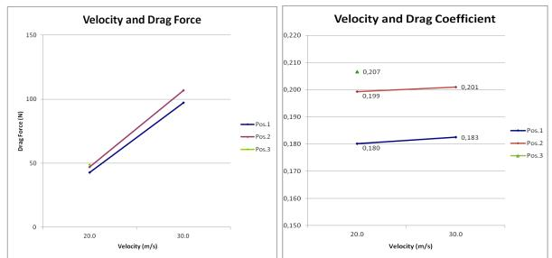
Figures 98 and 99 – Performance curves for D and CD according to test stages performed in 2010.
