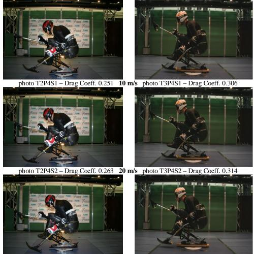
photo T2P4S3 – Drag Coeff. 0.296 30 m/s photo T3P4S3 – Drag Coeff. 0.322
