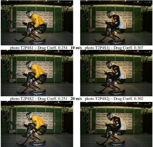
Figure 80: Position 4 – Extra Position & Position 5 – Extra Position using a jacket
