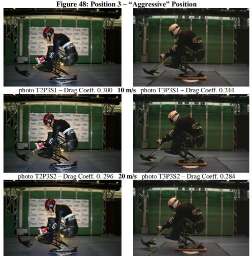
photo T2P3S3 – Drag Coeff. 0.303 **30 m/s** photo T3P3S3 – Drag Coeff. 0.283
