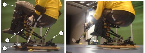
Figure 51: 1. Two parallel swings provide optimum shock absorption. Both pull and pressure are adjustable. 2. The binding plate perfectly simulates a ski boot, making it compatible with any make of binding. 3. Foot fairing and foot fairing cover for seat widths.
