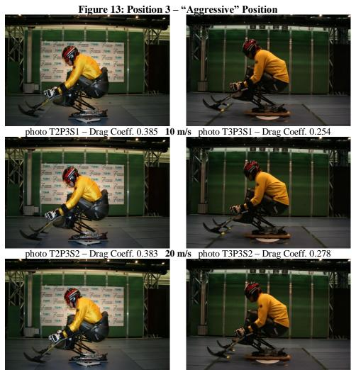
photo T2P3S3 - Drag Coeff. 0.300 30 m/s photo T3P3S3 - Drag Coeff. 0.300
