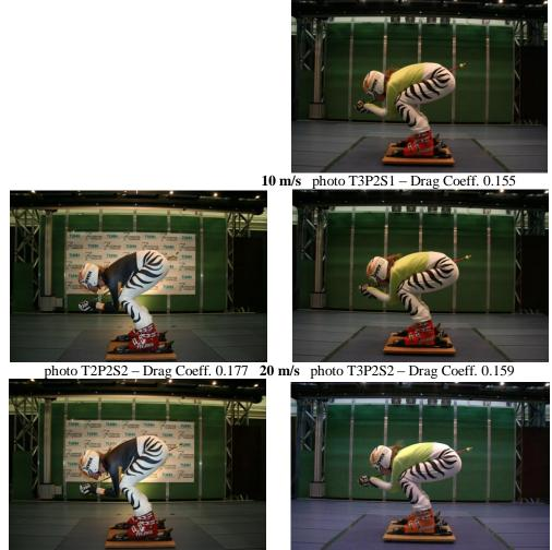
photo T2P2S3 – Drag Coeff. 0.186 30 m/s photo T3P2S3 – Drag Coeff. 0.157
