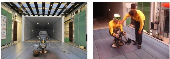
Fig. 20 (a, b): Frontal view from the test section; Seated mono-ski fixed to the balance.
