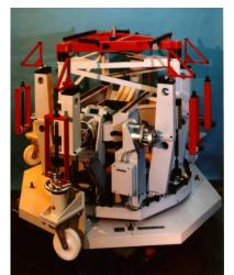
Fig. 22: Six-component (External) Balance (http://www.tu-harburg.de).
