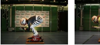
photo T2P1S3 – Drag Coeff. 0.178 **30 m/s** photo T3P1S3 – Drag Coeff. 0.184
