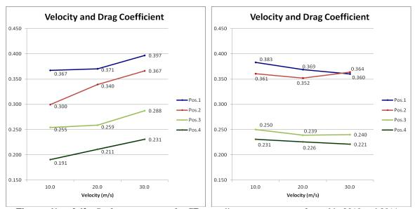
Figures 61 and 62 – Performance curves for CD according to test stages performed in 2010 and 2011.
