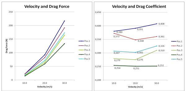
Figures 75 and 76 – Performance curves for D and CD according to test stage performed in 2010.
