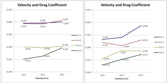
Figures 44 and 45 – Performance curves for CD according to test stages performed in 2010 and 2011.
