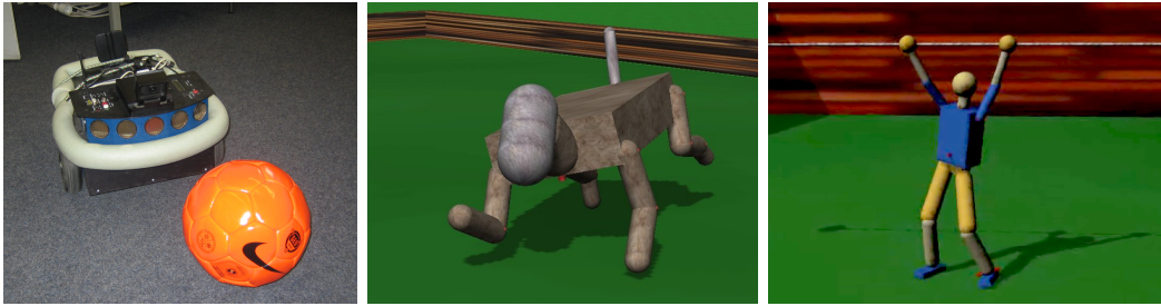
Figure 4.35: Other robots that have been controlled by the homeokinetic controller. Left: PIONEER robot [98] playing with a ball. Experiment conducted by Ralf Der and René Liebscher; Center: A simulated dog robot is learning to move; Right: Simulated humanoid robot performing athletic exercises. Videos can be found at [47].
