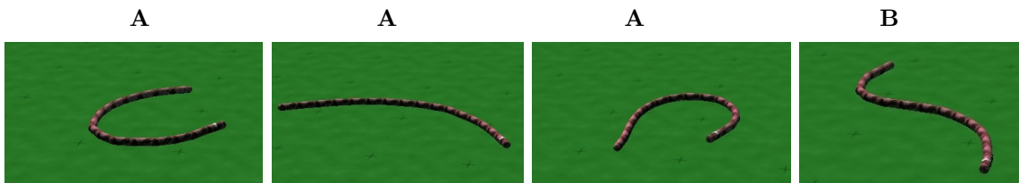
Figure 4.21: Main modes of the SNAKE robot The labels A and B correspond to the two principal components plotted in Fig. 4.20
