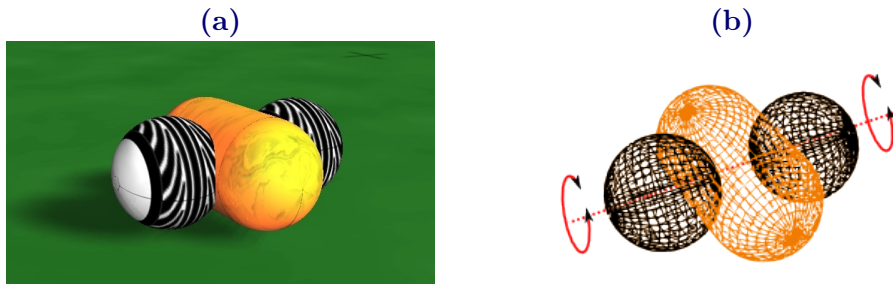
Figure 2.6: Pictures of the simulated TWO WHEELED robot. The robot has two actuated wheels and two wheel velocity sensors. (a) Screenshot taken from a simulation; (b) Wire-frame view with the axis of wheel rotation.
