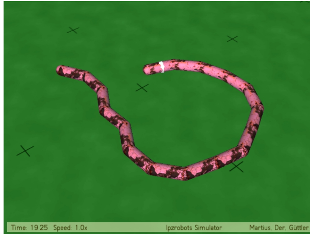
Figure 4.17: Planar SNAKE robot with 16 segments and 15 degrees of freedom. In this experiment it is fixated at the first segment with a joint (white ring) and has no friction with the ground.
