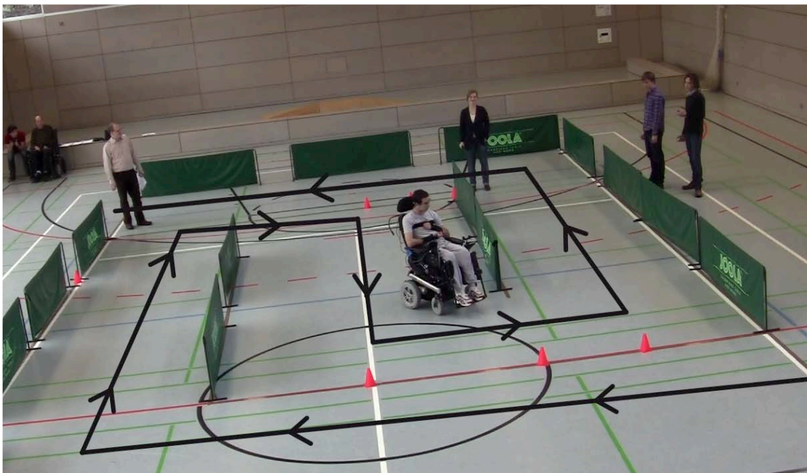
Figure 9) The real obstacle course for testing the performance of the ACS in subjects with tetraplegia.
