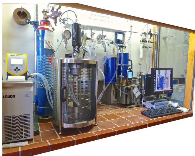
Figure 105: Foto of the reactor setup that was used for higher pressures.
