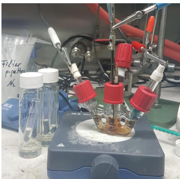
Figure 65. Typical CPE set up with the three electrode as compartmented via the sample holders. The additional septa on the sample holders are only used when long measurements are performed ( > 5 h) to prevent solvent evaporation.
