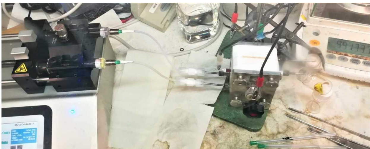
Figure 62. Flow cell set up with the syringe pump as used for initial attempts of electrochemical N_2 -splitting from \mathbf{1}^{Cl} . From left to right comes first the syringe pump with a solution of \mathbf{1}^{Cl} (purple, back) and a solution of Fc (yellow, front) in THF. The syringes are connected via PTFE tubes to the stainless steel entrances of the flow cell. The flow cell is connected via crocodile clamps to the potentiostat. After flowing passed the electrodes, the solutions are gathered in the attached vials on the right.
