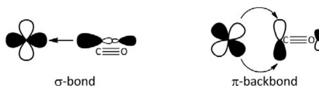
Figure 57 Synergistic bonding model of metal carbonyl complexes according to Dewar-Chatt-Duncanson.
