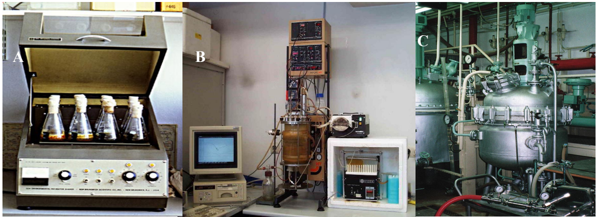
Plate 1. Submerged conidia production in liquid culture. A) Flask shaker culture, B) 3 L fermenter and C) 300 L fermenter.
