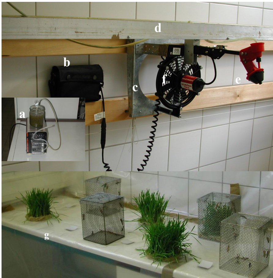
Plate 2. ULVAFAN-MK2 sprayer mounted on a run-way bridge for laboratory spray experiments. a) A liquid pump pumping OFC2 formulation and a rubber tube for delivery of the suspension into the sprayer tip, b) power supply for the sprayer, c) Sprayer holder, d) Run-way line support (front view), e) Sprayer tip, f) fan, g) sample plants and caged insects used during laboratory spraying.
