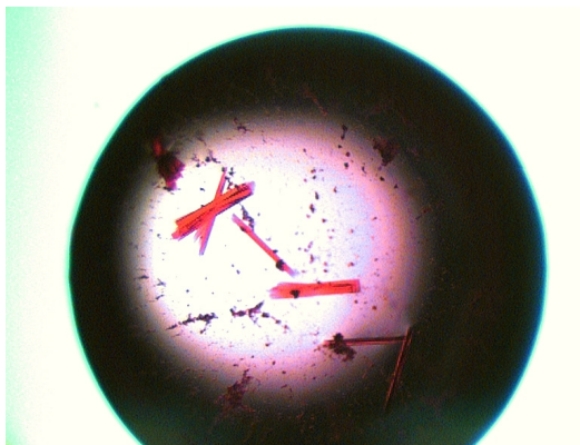
Fig. 3.5 Orthorhombic crystals of the 7-AAMD-TTAG[Br 5 U]T complex obtained with cross seeding.
