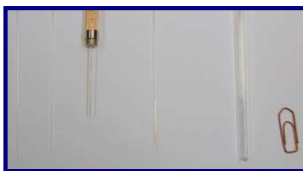
Figure 2.2: Open-ended glass capillaries of different dimensions. Comparisons of outer dimension 1.0 mm OD, 1.7 mm OD capillaries and thin-walled 5 mm NMR tube.
