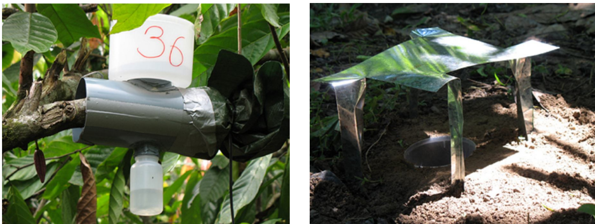
Figure 3.1 Trap system that was used for spider sampling within cacao agroforestry sites: brancheclector in a cacao tree canopy (left) and roofed pitfall trap (right).
