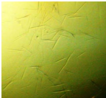
Figure 49. Needle like crystals grew during initial screening in conditions: Natrix nr. 33 (30 % Hexanediol, 0.2 M Ammonium Chloride, 0.01 M Magnesium Chloride, 50 mM HEPES pH 7.0), Crystal Screen 2 nr. 19 (2.5 M 1,6 Hexanediol, 0.1 M Sodium Citrate pH 5.6) and nr. 39 (3.4 M 1,6 Hexanediol, 0.1 M Tris pH 8.5 and 0.2 M Magnesium Chloride). The crystals were well reproducible over a relatively wide range of pH (7-10) and with different additives. No condition was found however that gave three-dimensional crystals and seeding attempts were not successful.
