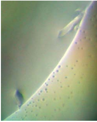
Figure 47. Crystals obtained in condition B6 of JBScreen 1 (30 % PEG 400, 0.1 M Tris pH 8.5, 0.2 M Sodium Citrate). The crystals were too fragile to be mounted on the rotating anode. Numerous attempts to reproduce the crystals failed.
