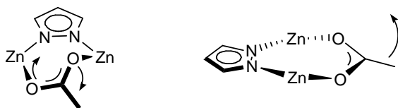
Scheme 2.13: Twisted (left) and tilted (right) binding motifs of the acetate ligand as it is reported in literature. [57]
