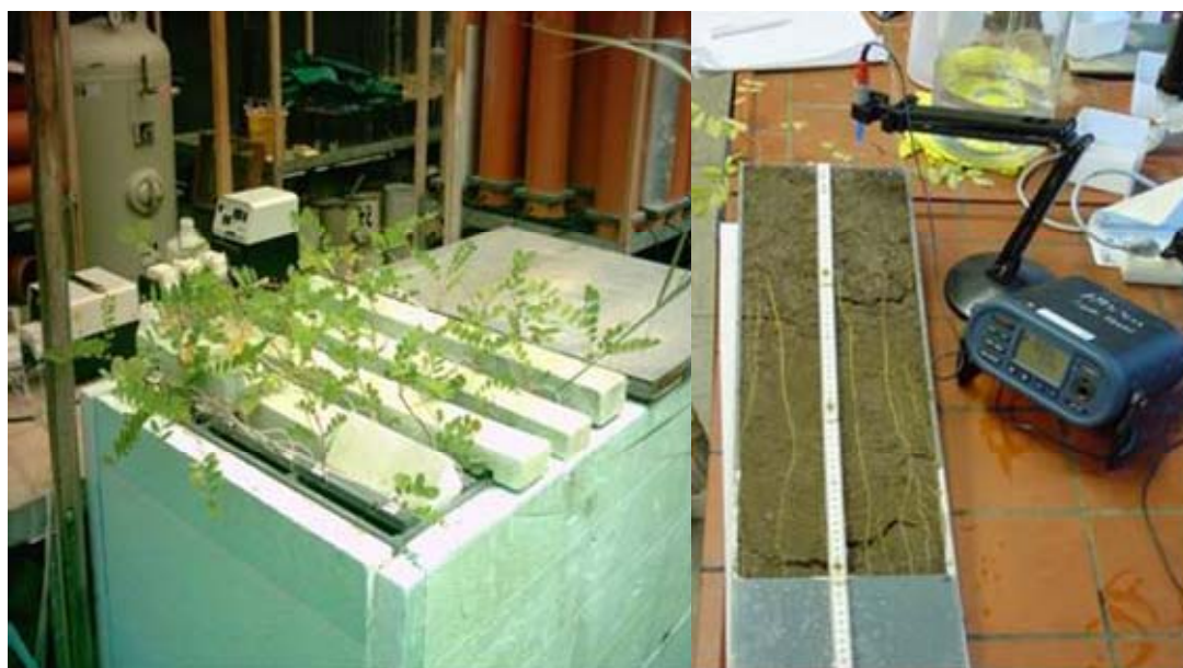
Figure 4.1: Arrangement of rhizotrons in the insulated wagon (left) and a rhizotron unit with two single rhizotrons (right).
