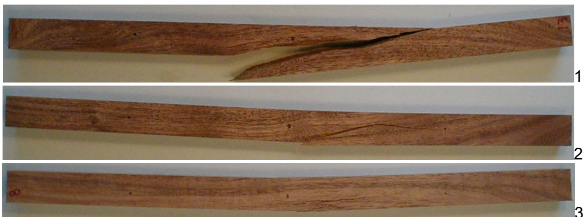
Fig. 35: Type of failures in static bending of P. laevigata wood according to ASTM 143-94. 1 and 2 are typical failures from cross-grain tension and 3 from wood tension.
