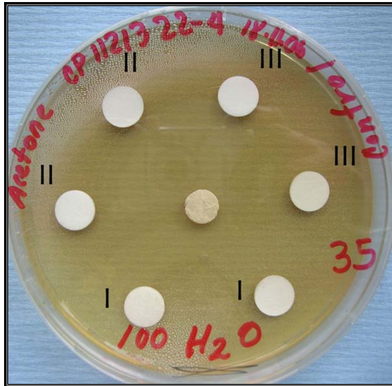
Fig. 40: Distribution of cellulose discs in petri dish (diameter 140 mm): I) cellulose discs impregnated with P. laevigata extractives, II) cellulose discs impregnated with acetone (acetone control), III) cellulose discs not impregnated (control discs). The circle in the center corresponds to the fungus.
