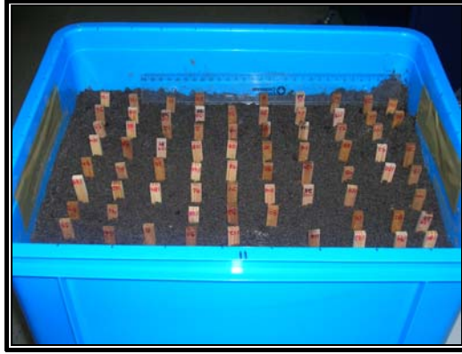
Fig. 36: Plastic container used to expose P. laevigata test specimens to unsterile soil.
