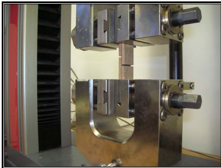
Fig. 47: A general view of tensile shear test according to EN 302-1; Zwick/Roell Z100 testing machine.
