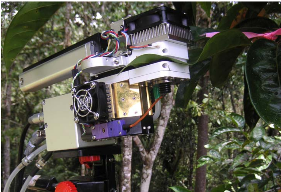
Figure 1.3. Leaf chamber of photosynthetic gas analyzing apparatus Licor 6400
