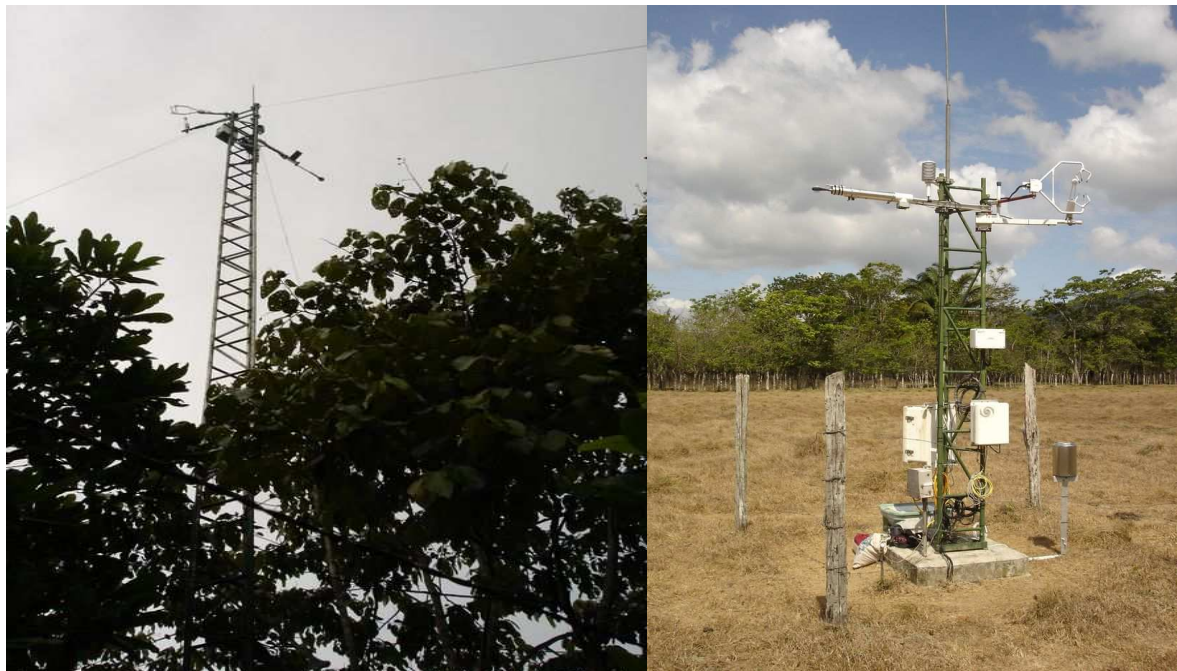
Fig. 10: Eddy flux towers in the center of the plantation and on an adjacent pasture. Micrometeorological measurements were conducted by Sebastian Wolf (photos: Sebastian Wolf).
