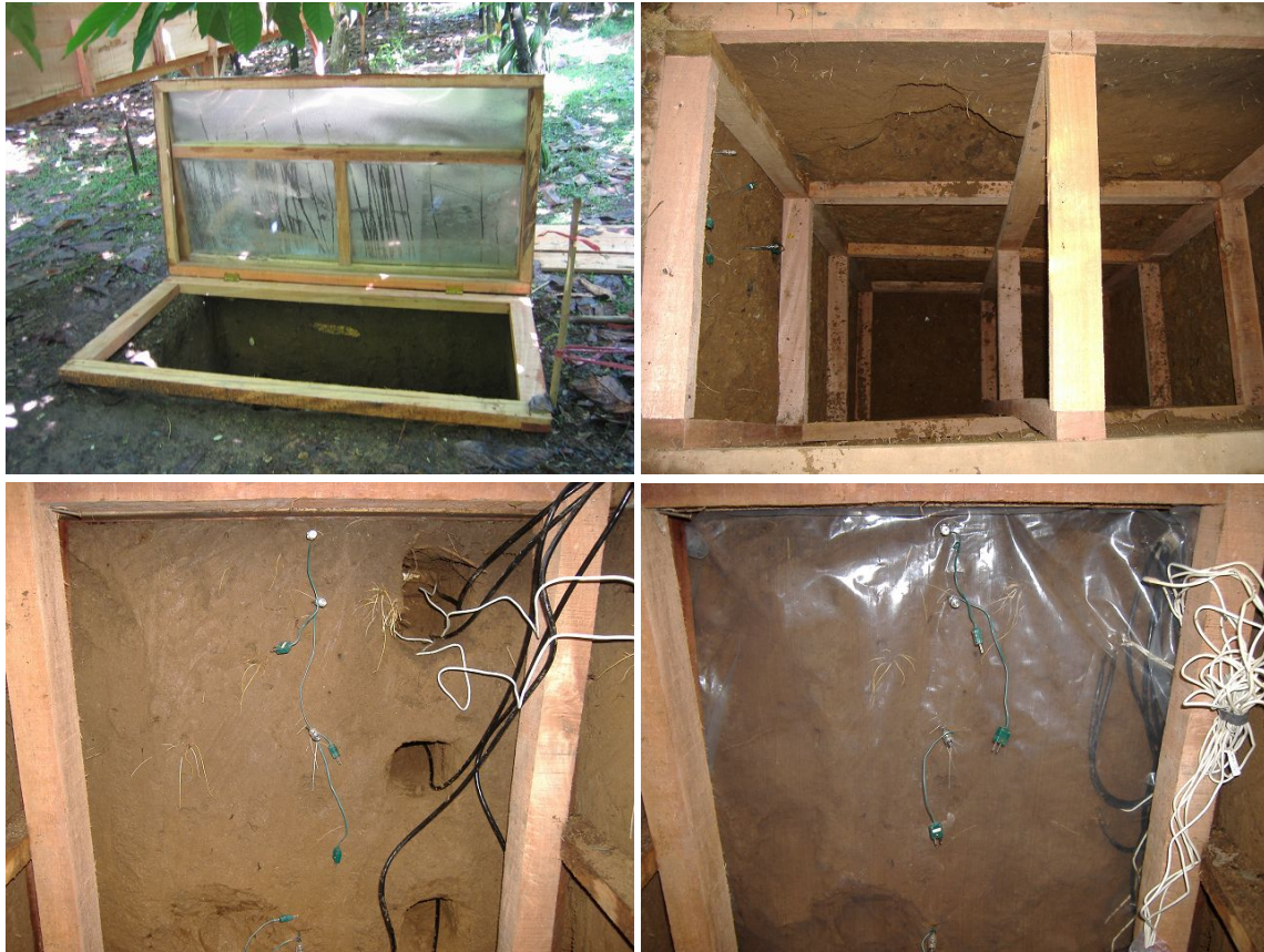
Figure 8: Soil pit lid (Picture by Oliver van Straaten), view into the pit, TDR installation into the pit walls and plastic covered pit wall. The black wires denote to TDR and the white and green ones to other installations
