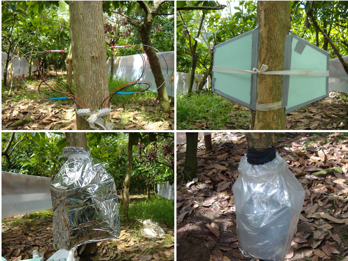
Figure 7: Installed sap flux sensor, shielding with Styrofoam, reflective foil and plastic.
