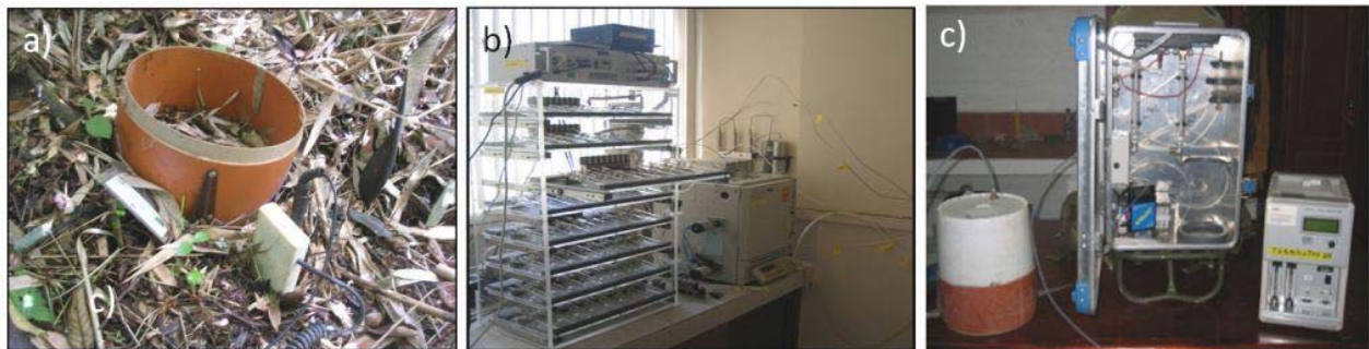
Figure 1.3: Field and laboratory equipment for soil trace gas flux measurements. a) Chamber base for static and open dynamic chamber measurements with thermometer and hydrometer for concomitant temperature and soil moisture measurements, b) gas chromatograph with autosampler and glass vials for the measurement of \text{CO}_2 , \text{N}_2\text{O} and \text{CH}_4 , and c) LMA-3D \text{NO}_2 Analyzer for NO measurement with the closed chamber. Photographs: Katrin Wolf and Guntars O. Martinson.
