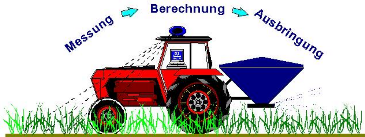
Abb. 4: Konzept des Hydro N-Sensors (© HydroAgri, URL: http://www.hydroprecise.com/index_ger.htm [09.05.02])
