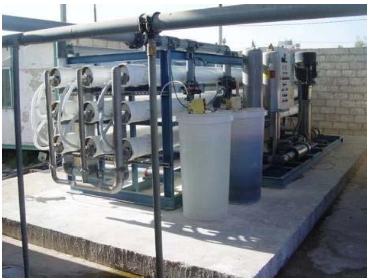
Fig. 3-7: Privately owned desalination plant in South Shuneh. Brackish well water is desalinated. Desalinated water is mainly used for irrigating banana farms.
