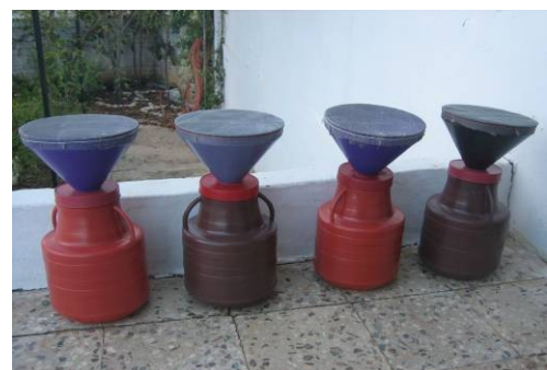
Fig. 4.14b: Manual built supportive rain gauges for data accuracy.
