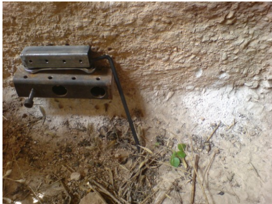
Fig. 5.10: The mortar powder spilled during installation can still be seen at the end of the water year 2007/2008 (in one of the monitored subwadies).
