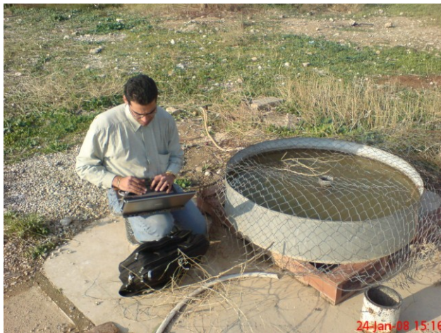
Fig. 5.8: Class A land pan used to calculate the evaporation from the reservoir.
