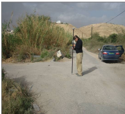
Fig. 4.2a: Taking a GCP measurement in Jordan Valley using Differential Corrected GPS measurements.
