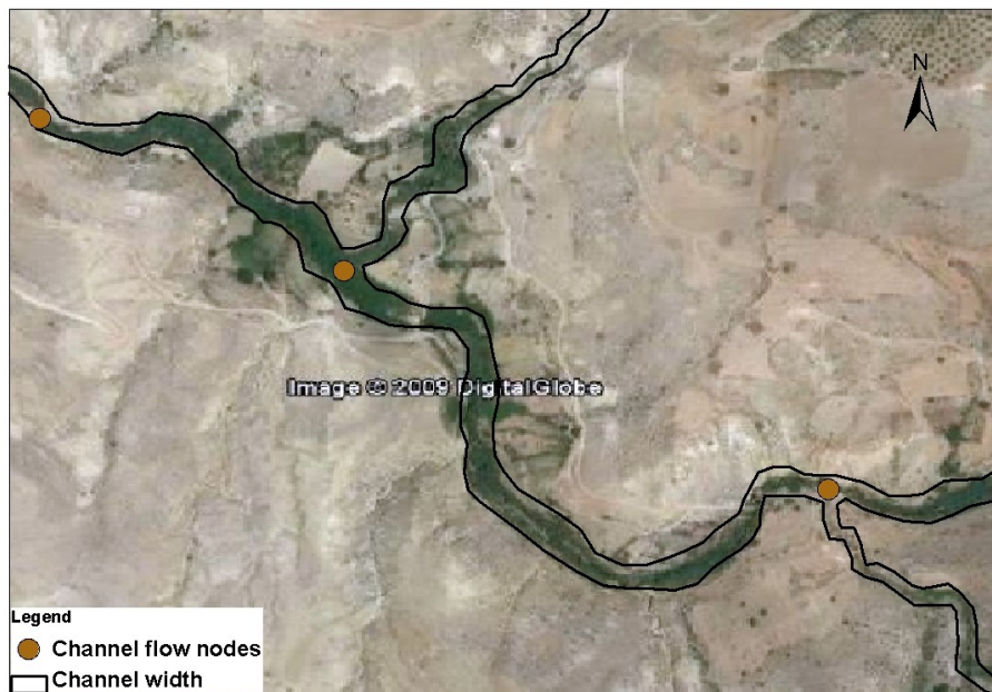
Fig. 5.35: Calculation of the spatially averaged channel width (background image from Google Earth®).
