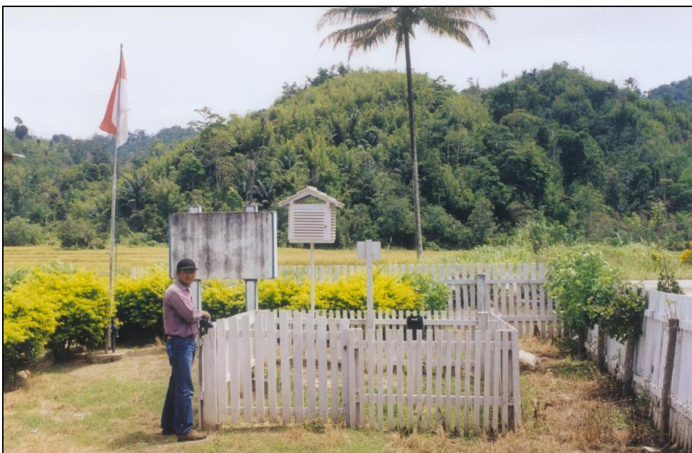
Appendix A. 4: Tongoa climate station equipped with a precipitation pulse transmitter and a two channel datalogger for air temperature and humidity.
