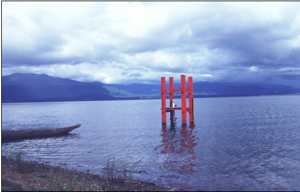
Appendix A. 3: Lake Lindu gauging station equipped with a float operated shaft encoder with integral data logger.
