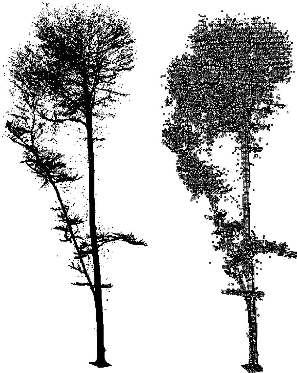
Fig. 2: Three-dimensional point cloud of a single tree as created by the scanner (left). Voxel-based representation of the same tree as used for the calculation of structural parameters with Mathematica based on voxels of 10\text{ cm}^3 volume (right).
