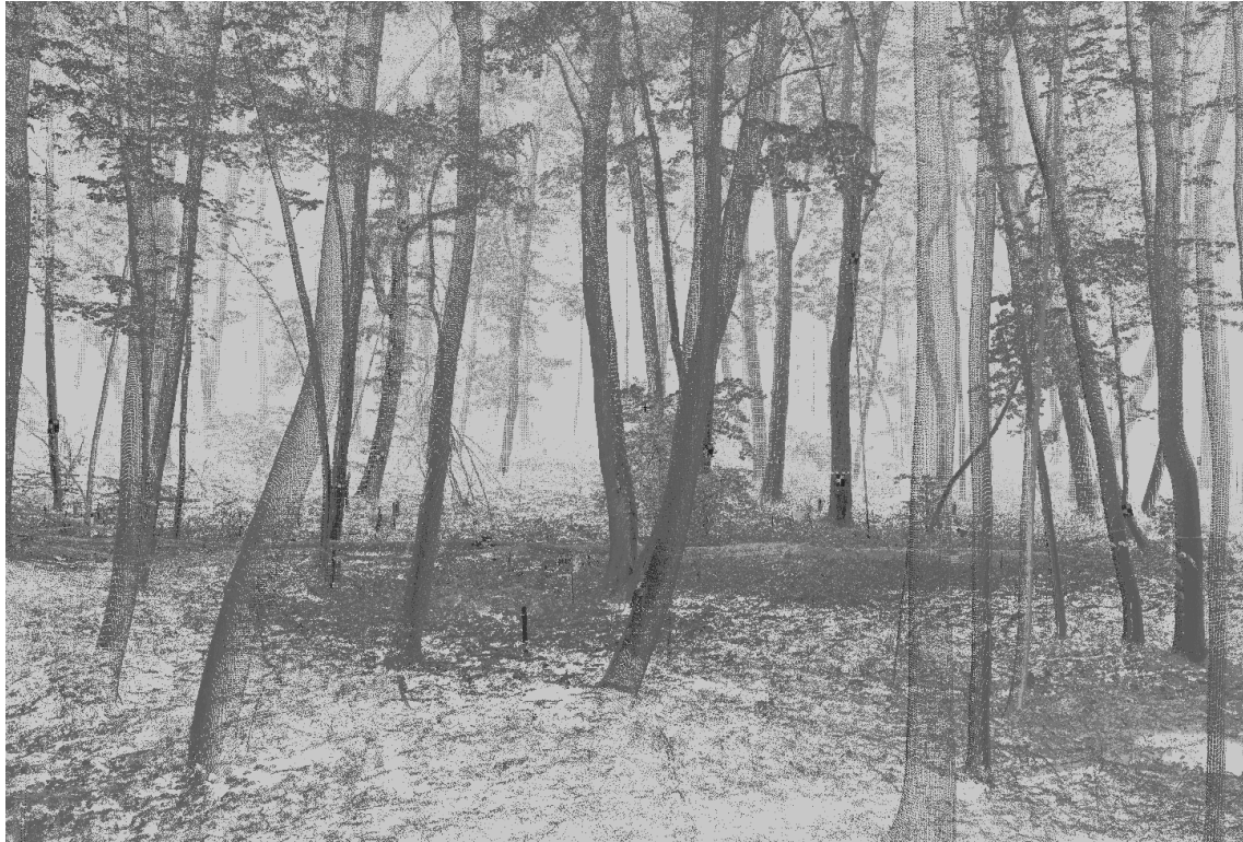
Fig. 2: Exemplary point cloud of a tree cluster and its immediate vicinity, based on six scans ( 10^6 points).
