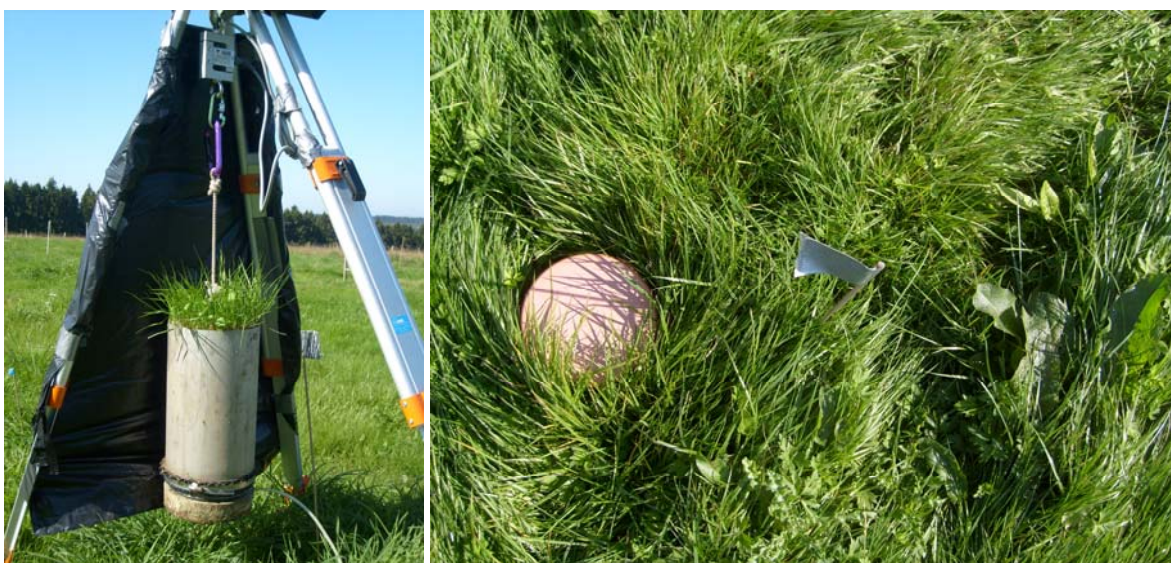
Figure 8.5: Weighing of lysimeters and lysimeter within the sward as described in Chapter 4.
