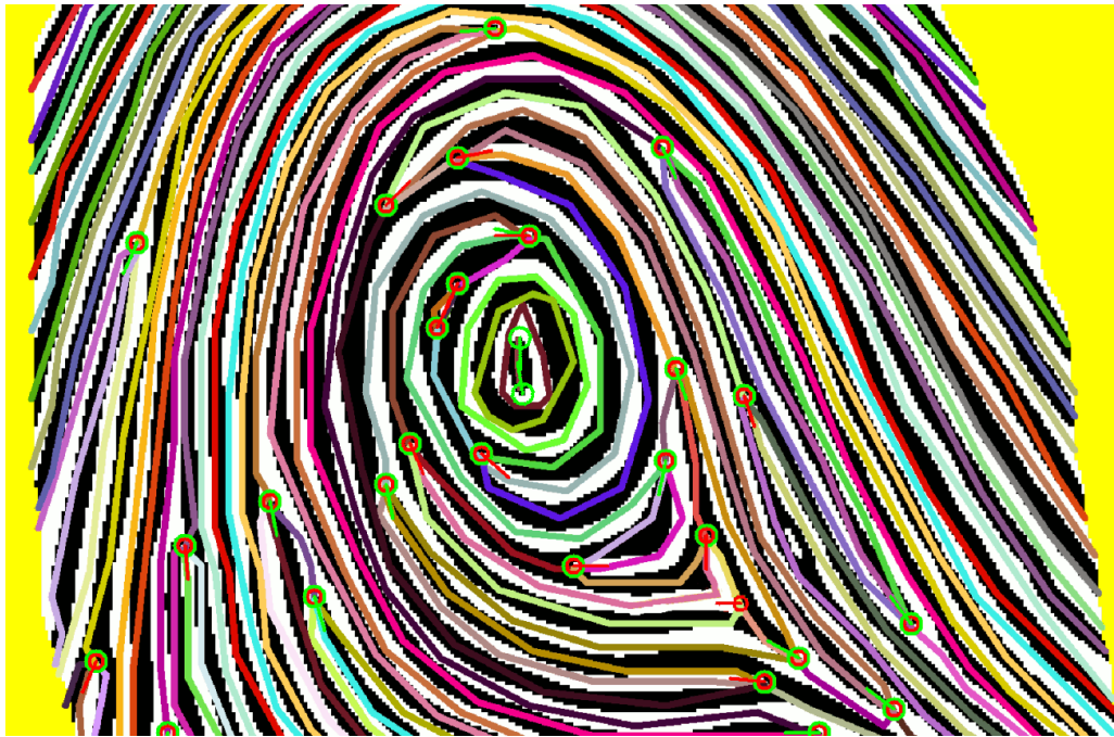
(a) Fingerprint structure with underlying binarised image. Each segment is marked with a different colour. Endings are marked in green and bifurcations in red. Note the unvalidated minutiae at the core points where only endings and no bifurcation are marked and at the delta point where a bifurcation but no ending is marked.
