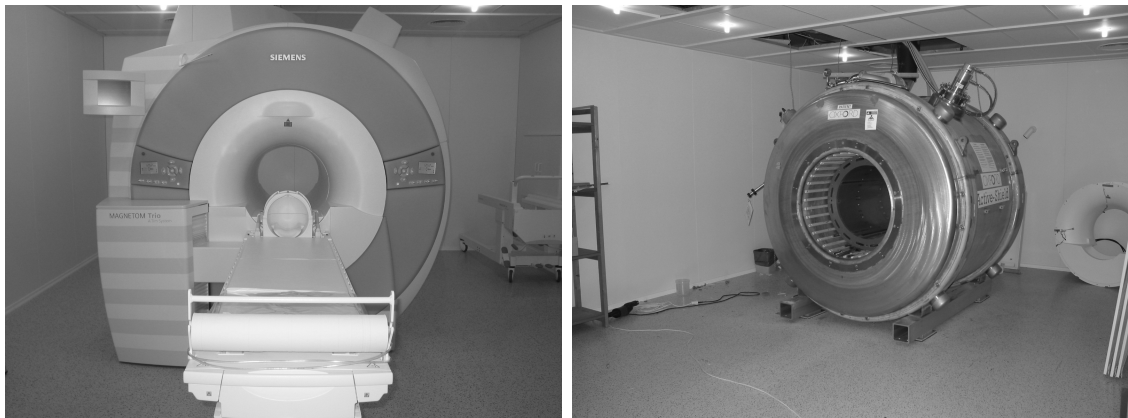
Figure 4.1: Whole-body MRI system: (left) with and (right) without housing.
