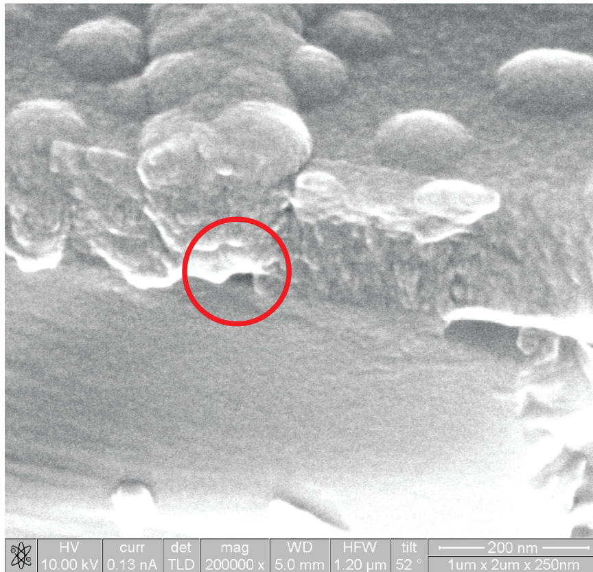
Figure 2.3: Scanning electron micrograph of a single channel waveguide exit (red circle) after cutting but still unpolished.
