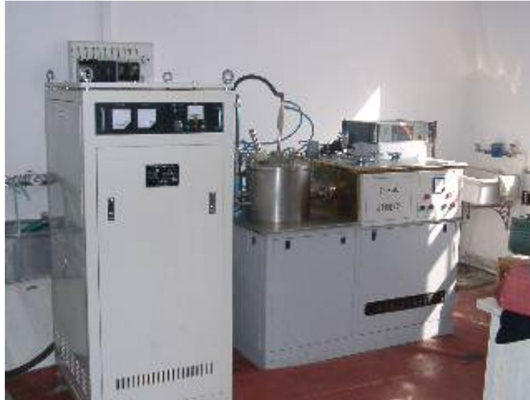
Figure 3.1 Vacuum arc melting furnace for Cu mould suction casting in Department of Materials Engineering, Dalian University of Technology, Dalian, P. R. China 2 .
