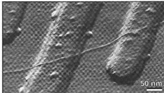
Figure 7.3: AFM picture of a carbon nanotube on top of a Si/SiO 2 substrate with Pt electrodes. The electrode in the upper left corner is used to change the electrostatic potential of the nanotube via an applied gate voltage. A bias voltage is applied between the other two electrodes. Reprinted by permission from Macmillan Publishers Ltd: Nature 386 , 474, copyright 1997.
