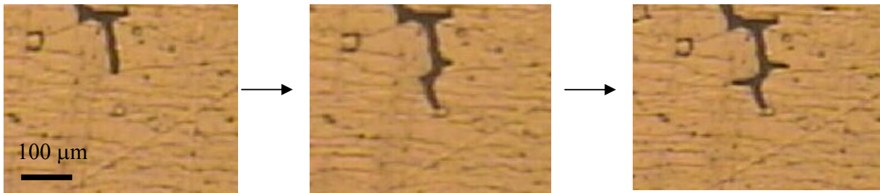
Figure 3.24: buckle growth of a Pd20nm/Nb100nm/Pd20nm film on 1mm PC by growth of a new buckles perpendicular to the existing buckle and divided it on a half length.
