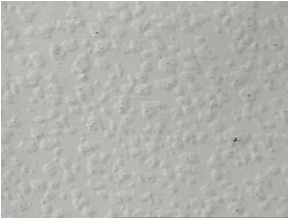
Figure A.2: Light microscopically images of the surface morphology change during hydrogen loading of 2.5\mu\text{m} Nb-layer on 0.2\text{ mm} sapphire substrate.
