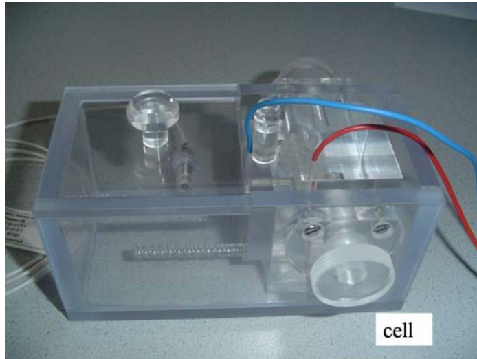
Figure 2.4: The second cell for controlled hydrogen loading, prepared for exhibition during Hanover Trade Fair 2006. The blue wire is for the contact with a sample, the red wire is contacted with the counter electrode.
