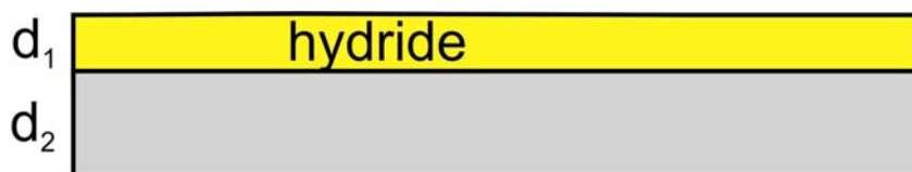
Figure 3.18: Schematical drawing of a sample with hydride formed in the upper layer of thickness d_1 .
