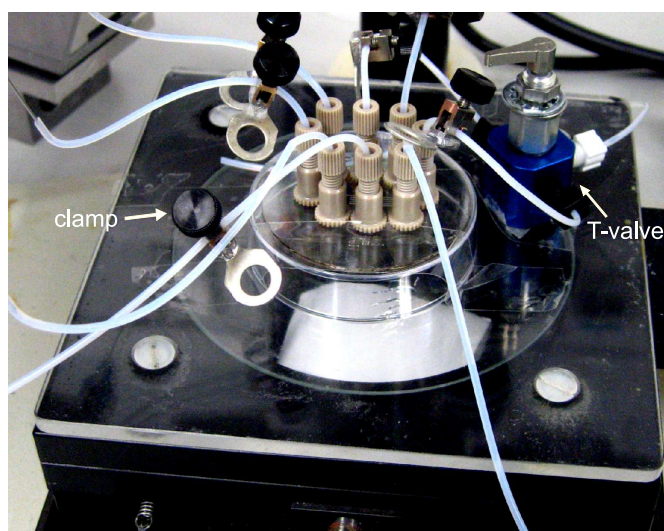
Figure 5.2: Experimental set-up with the microfluidic chip, t-valve and small clamps used in the experiment.
