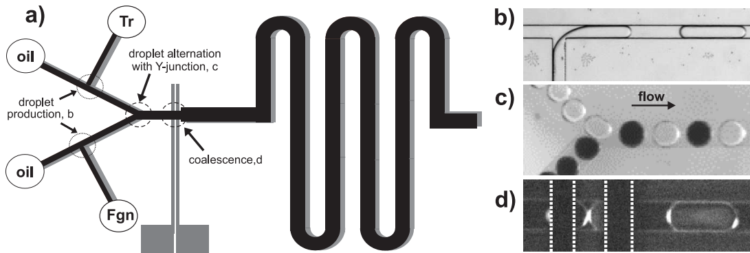
Figure 6.2: a) Microchannel design with 4 inlets. b) Droplets of thrombin (Tr) and fibrinogen (Fgn) solutions form at T-junctions. Droplets alternated b) at the Y-junction and d) coalesced when electric field is applied (electrodes marked with dashed lines).
