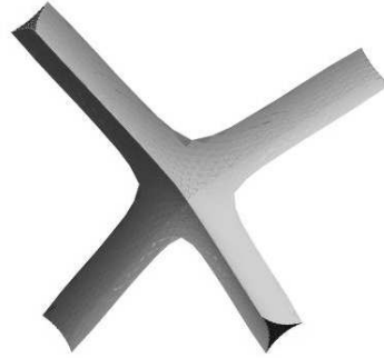
Figure 1.4: The elementary Plateau border junction in three dimensions. Image taken from Ref. [90].
