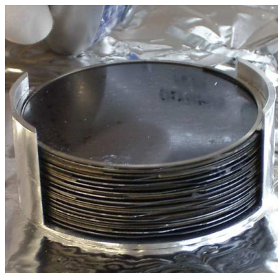
Figure 4.10: Photo of a typical 'sandwich sample': 20 silicon wafers, each supporting several hundreds of highly oriented phospholipid bilayers are placed on top of each other in an aluminum frame, separated by a pair of aluminum spacers. This allows the D_2O -vapor to flow between single wafers.
