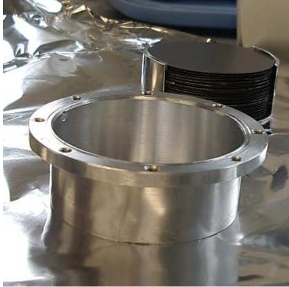
Figure 6.6: Photo of sample-assembly: the sandwich-sample visible in the background is inserted into the aluminum container visible up front. Then the liquid mixture containing 2 wt% PEG 20000 solved in D_2O as well as deuterated Ethanol d-6 is carefully pipetted inside. The container lid is sealed at the top with indium wire and eight screws.
