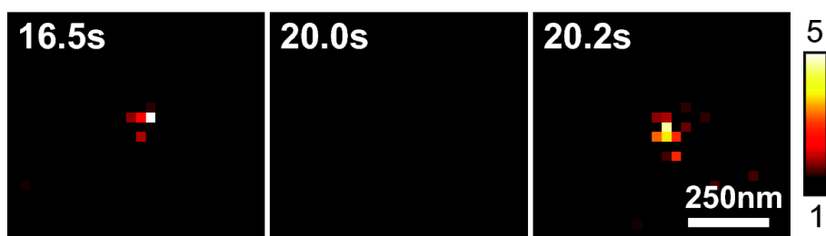
Figure A.2: Blinking in fixated samples. Occasionally vesicles which were visible in a succession of frames (left panel) disappeared instantly from one frame to the next (middle panel), only to reappear after up to a few seconds (right panel). This behavior, termed blinking, is known from single molecules and few-chromophore systems and was also occasionally observed in standard confocal fluorescence recordings.
