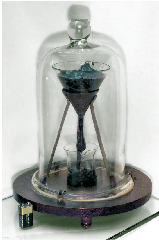
Figure 1.14: Pitch drop flowing through a funnel, University of Queensland in Brisbane, Australia.
