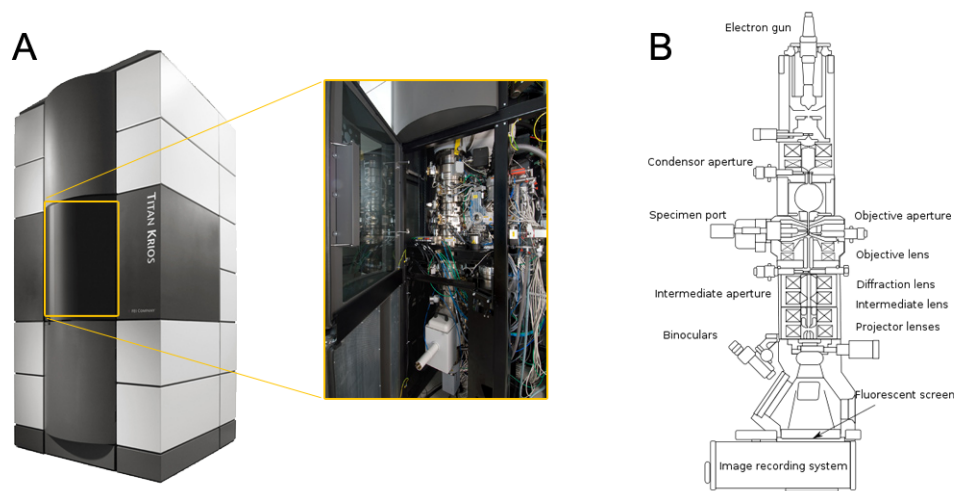
Figure 1.2: A: The latest generation of a TEM, the FEI “Titan Krios”. The overlay (indicated by the yellow frame) shows the microscope as it would look like with front doors open. B: Schematic illustration of the main components a TEM is built of.
