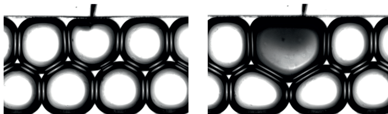
Figure 1.8: Addressing a single droplet with a pipette
