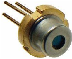
Fig. 2.14: a.) 5.6 mm closed can laser diode b.) Basic structure of a semiconductor laser diode assembly. Beam ellipticity is caused by the asymmetric geometry of the emitting active layer.
