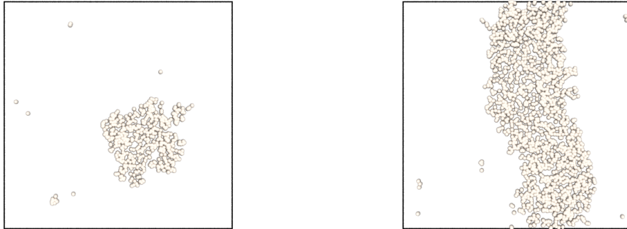
Figure 5.1: The two possible shapes that the minority phase can assume in a two-dimensional system are the droplet shape shown in the left and the slab shape shown in the right image.
