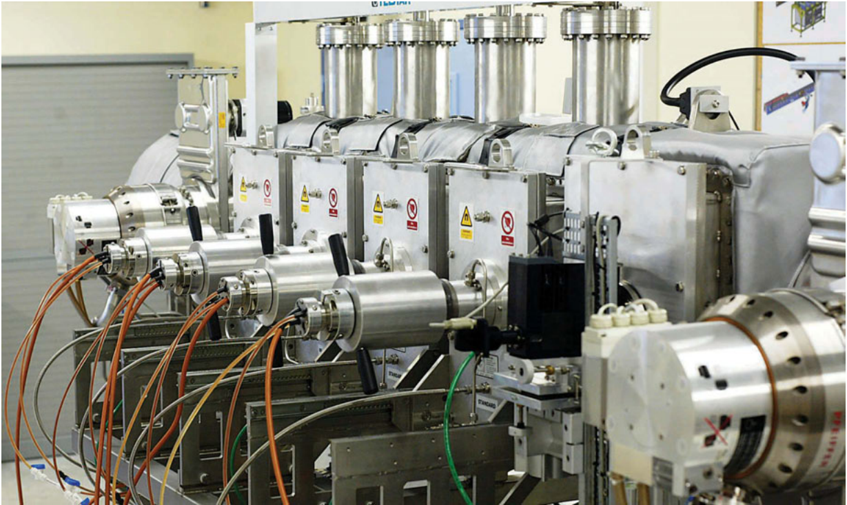
Figure 4.3: Photograph of the magnetron sputtering machine in the multilayer laboratory of the ESRF. Visible are the four cathodes and the long vacuum chamber.
