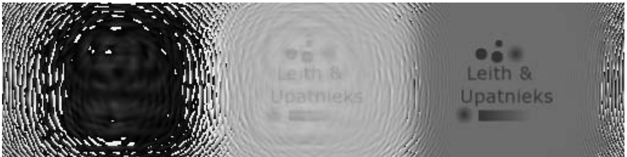
(d) Phase of the reconstructed wave: The reconstructed first order object wave (right) is evidently of much higher quality than the conventional Gabor hologram (zeroth-order beam, middle) and allows for a clearer identification of objects with fuzzy edges in particular. Due to the different propagation direction, the first-order beams are modulated in the horizontal direction by a term \exp(\pm ik\theta x) . For better visibility, this term is eliminated by taking the averages over one period 2\pi/k\theta .
