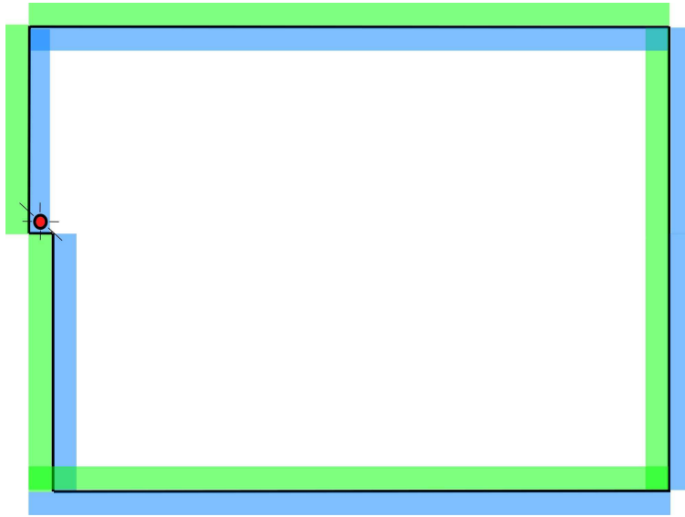
Figure 3.5: Schema of boundary conditions for our matrix of changeable size. Points, which are located on the colored strips inside the matrix are copied to the correspondent colored strip outside the opposite side of the matrix. The red circle represents the edge point on the matrix, where lipids, removed after creating a pore are inserted ( and lipids, needed to destroy a pore are taken from ). Black lines represent interactions with nearest neighbors ( 6 in case of hexagonal lattice ). This number of point in the last row of the matrix ( where the red point is) can change, while creating or destroying the pores. As well the number of rows can change, when the end this last row is reached by the red point.
