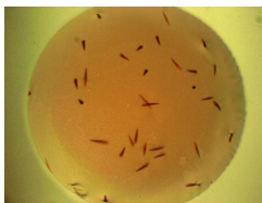
Figure 3.1. Red needle-shaped crystals with a length of 100 \mu\text{m} of the trioxacarcin-d(CGTACG) complex.
