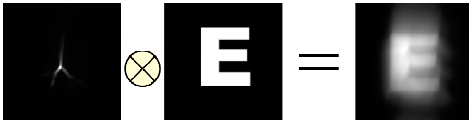
Figure 1-2 The convolution of an object in this case the capital letter E and an aberrated PSF in this case the PSF of a human eye. Figure modified from (Yoon, Jeong et al. 2004)
