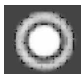
Figure 1-3 The PSF for a perfect optical system is the Airy disc, which is the Fraunhofer diffraction pattern for a circular pupil.
