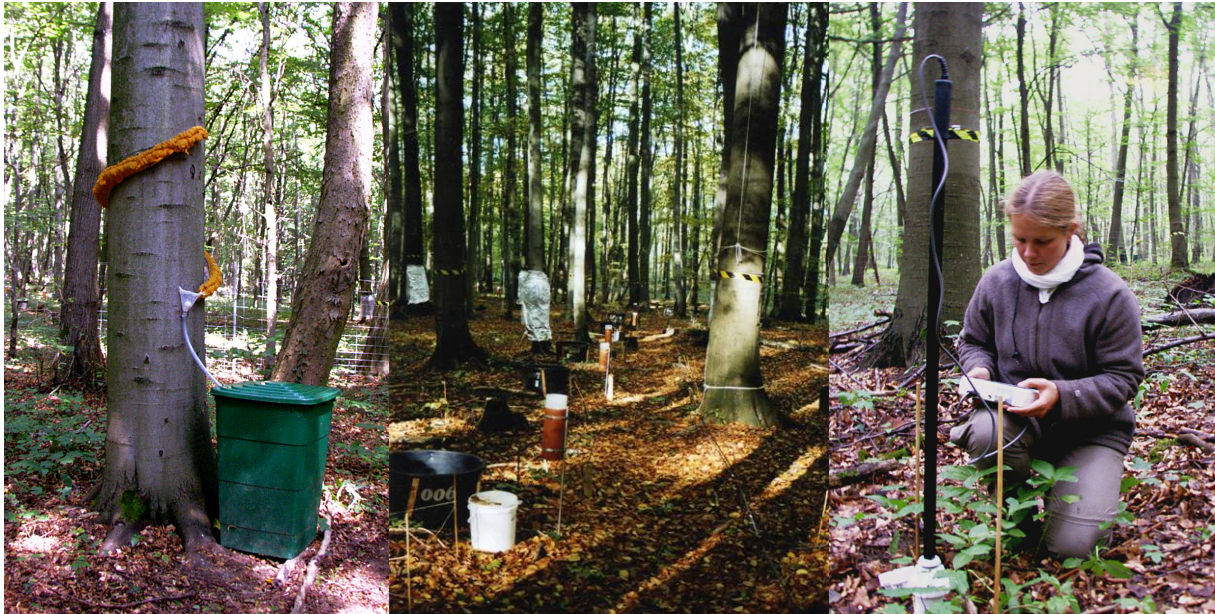
Figure 1.4 Measurements of stemflow, throughfall, and soil water dynamics (FDR technique) in the present study.
