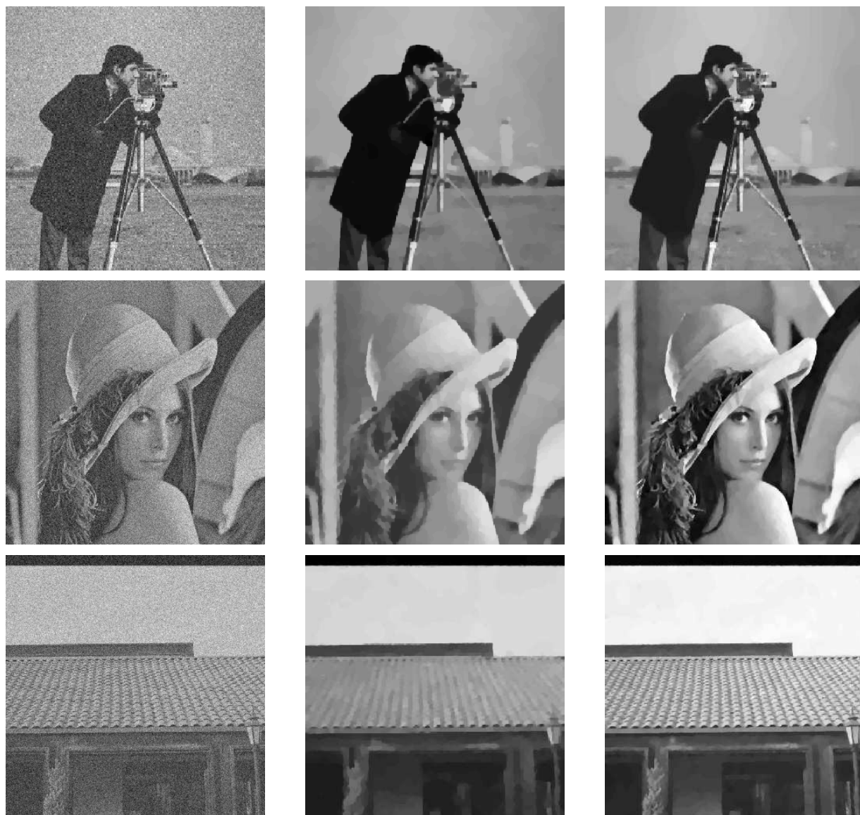
Figure 4.10: Global reconstructions and SMR-estimators. Left: noisy data Y = u + \sigma\varepsilon with \sigma = 0.1 . Middle: global TV -penalized least-squares reconstruction \hat{u} . Right: SMR-estimators \hat{u}_N(0.9) .
