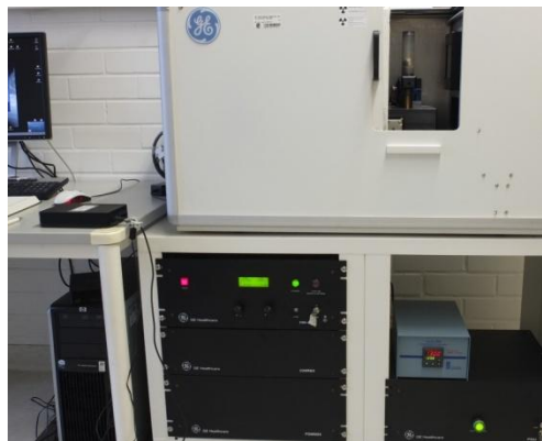
Abb. 4.3: Micro-Computertomograf, eXplore locus SP micro-CT (GEHC, Ontario, Kanada)
