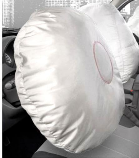
Figure 6.1.: Wrinkles in an inflated airbag.
