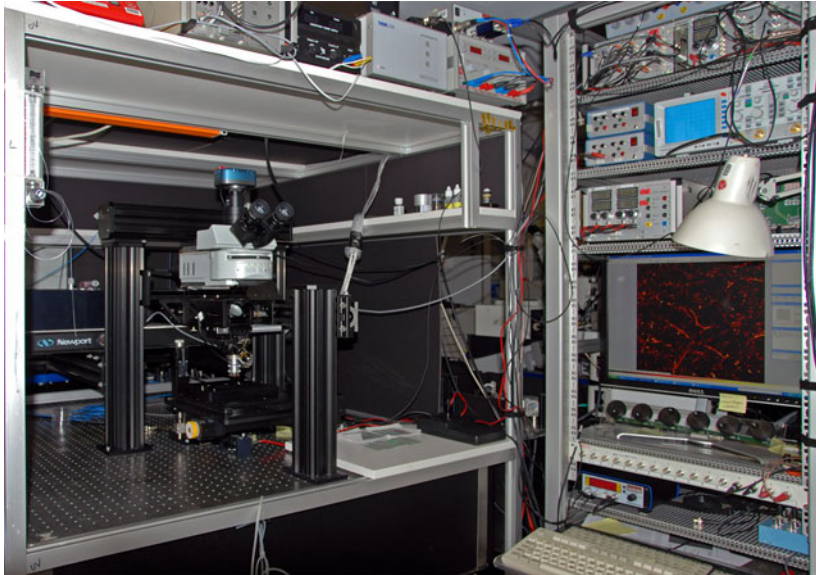
Fig. A.2.1: Overview of the complete laboratory setup built for in-vivo STED microscopy in this thesis. The PC on the right controls image acquisition. Lasers and optics for beam conditioning and fiber coupling are not depicted.
