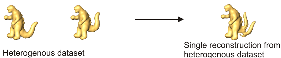
Figure 1.8: Averaging of a conformationally heterogeneous dataset leads to falsified images. Image courtesy of Florian Hauer.
