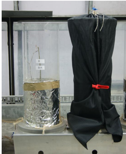
Fig. 4.1. The soil columns made of acrylic glass used in the experiments (50 cm in height and 17 cm in diameter). Left, non-shaded (normal situation) and right, shaded columns (during gas flux measurements) are shown. Courtesy of Marco Gronwald.
